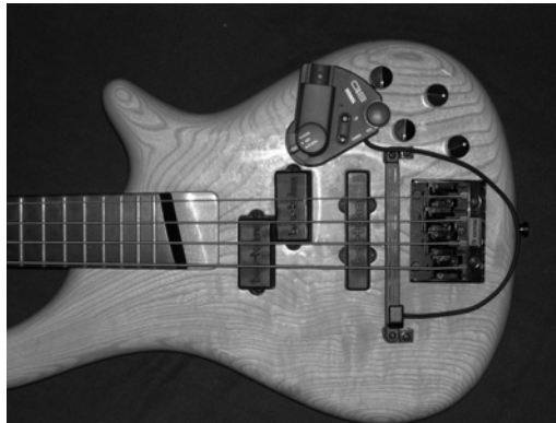
Figure 2.16 A Yamaha bass to MIDI converter in the 4 strings configuration (Courtesy of Yamaha).
