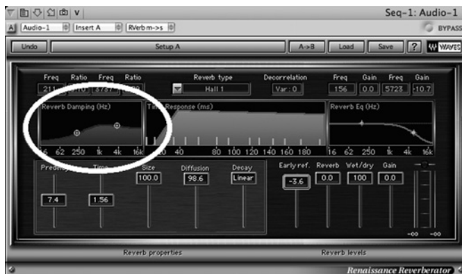
Figure 2.28 Use the damping parameter of your reverb to apply reverberation only to the higher frequencies of a drums/percussion mix (Courtesy of Waves).
