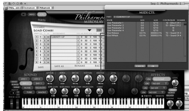
Figure 4.27 Example of CC#72 and CC#73, the release and attack of a clarinet patch in IK-Multimedia Philharmonik (Courtesy of IK-Multimedia).
