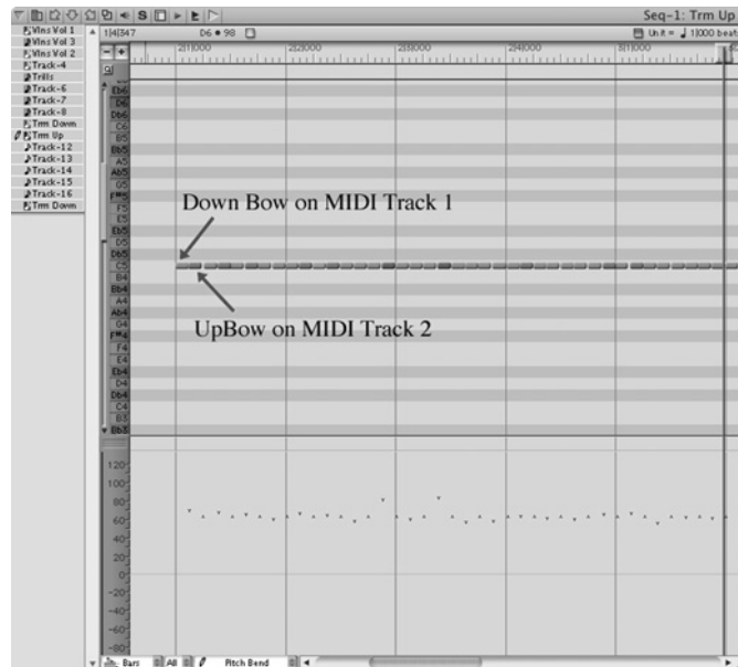
Figure 3.37 Tremolo effect: two different patches on two different MIDI channels alternating using the up/down-bow technique (Courtesy of MOTU).
