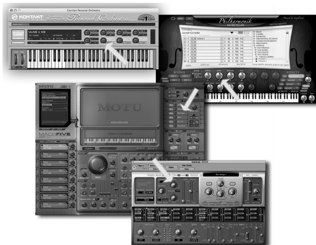
Figure 3.38 Some examples of the detune parameters in some of the most common sample-based orchestral libraries (Courtesy of MOTU, Garritan, Apple Inc., and IK-Multimedia).
